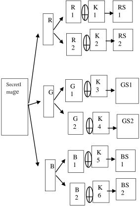
Fig2: Operation procedure to produce R,G,B shares.
